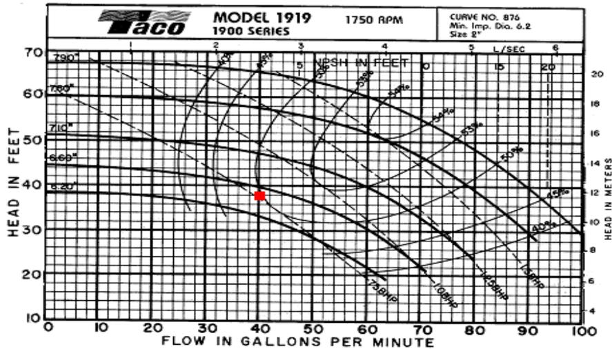
**Figure 2, Taco 1919 Pump Curve**
