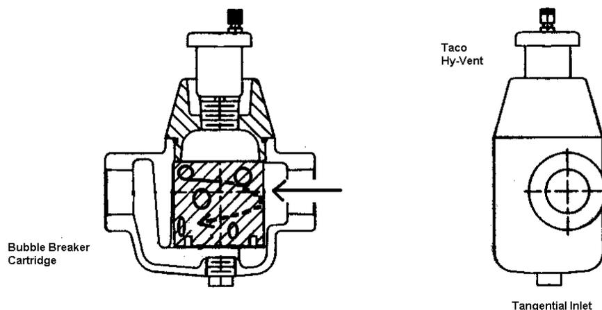
through holes at the bottom of the cartridge, and exits on the side opposite the inlet. At this time Vortech units are available only in ¾” through 2” sizes. They can be used in air separation or air control systems.
