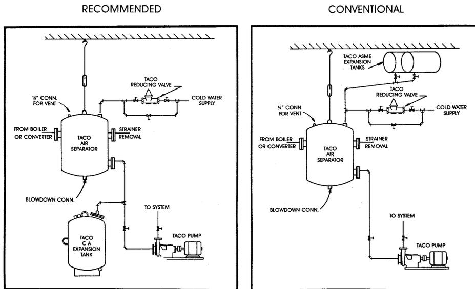
*Commercial Air Separators in Air Elimination and Air Control Systems*
