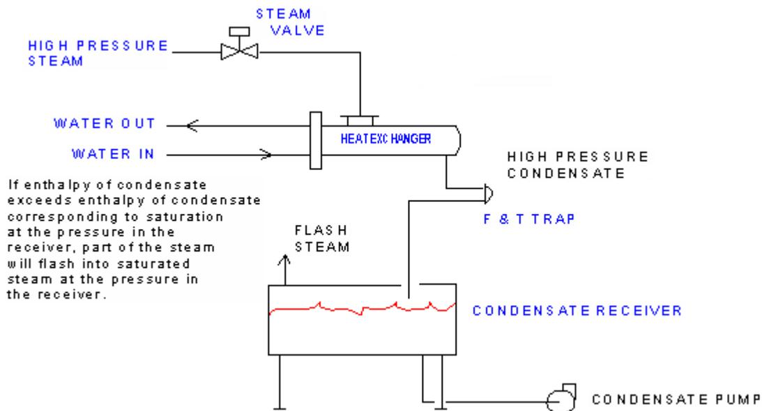
Figure 4, Typical Application Resulting in Flash Steam
