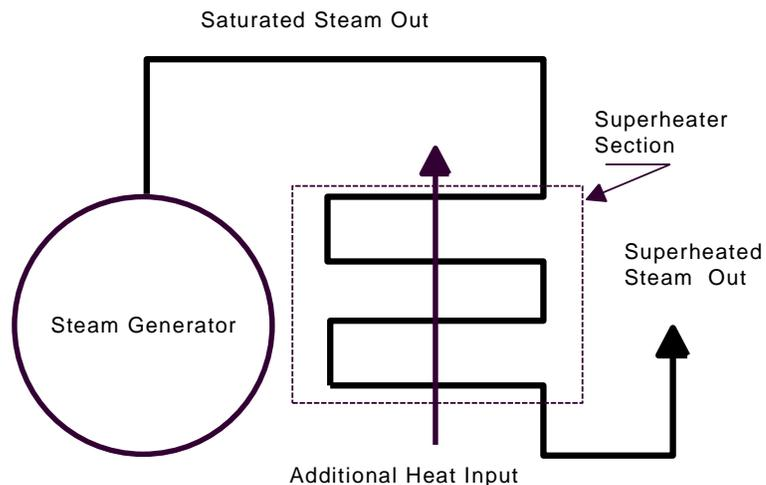
**Figure 3, Boiler With Superheater**
