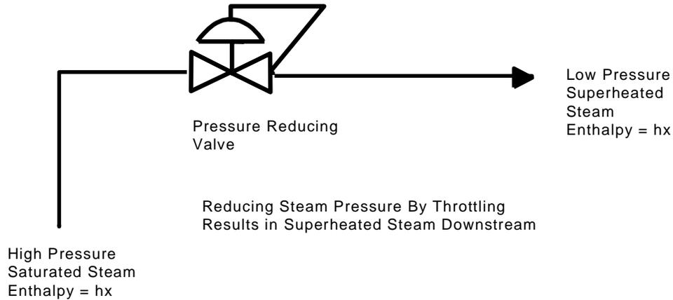
**Figure 5 Steam Pressure Reducing Schematic**
