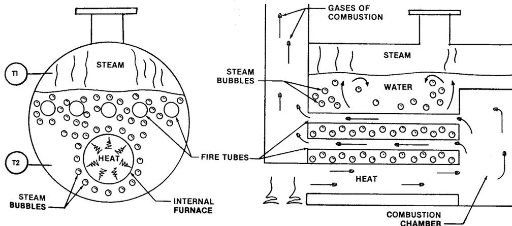
**Figure 1, Typical Fire Tube Steam Boiler**
